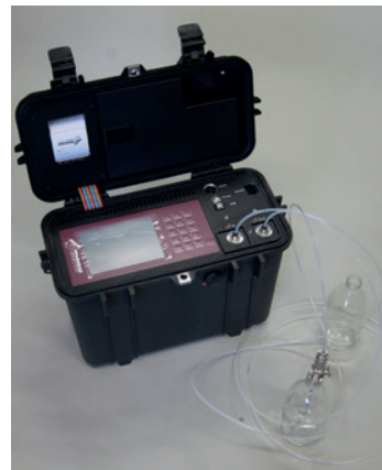
For batch sampling, the PAMAS S40 GO AVTUR is equipped with a sampling probe.
